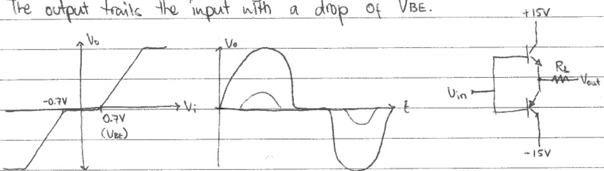
It can be alleviated with FEEDBACK (op-amp) or biasing the push-pull follower with diodes & resistors:
