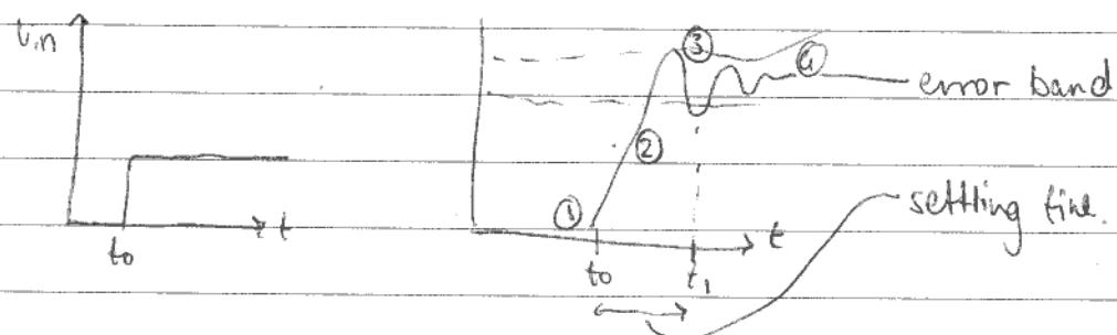
Settling time includes delay to the onset of output slewing ① and slewing time ② and recovery time from slew over load ③ and finally settling in the error band
